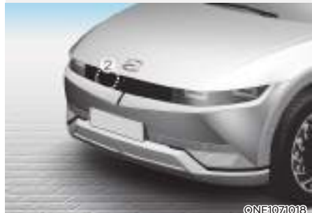
[1]: Front view camera, [2]: Front radar
