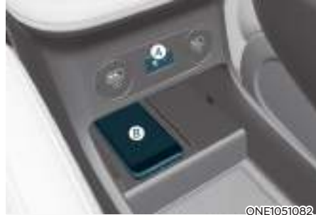
[A] : Indicator light, [B] : Charging pad
